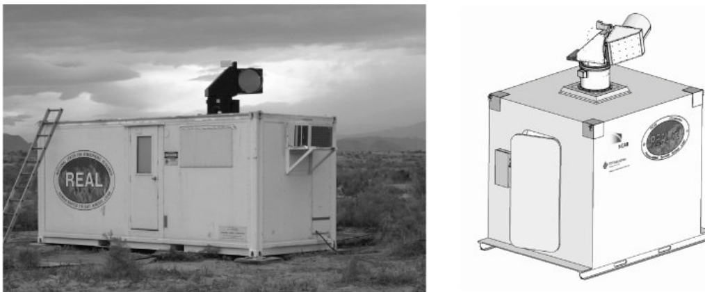
Figure 1: Left: Photograph of the field deployable REAL v1 at Dugway Proving Ground in October of 2004. Right: Drawing of REAL v2 that is currently in continuous and unattended operation from a permanent location in a major city for the surveillance of aerosol plumes.
