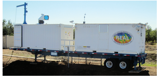
Figure 2: The NSF/NCAR Raman-shifted Eye-safe Aerosol Lidar (REAL) at California State University Chico.
