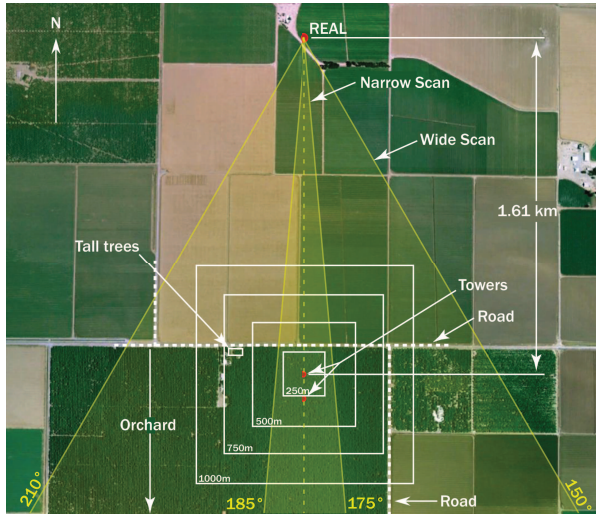
Figure 3: The NSF/NCAR REAL was located exactly 1.61 km north of a 30-m tall tower during the 2007 CHATS field experiment near Dixon, CA. 2-component wind vectors were calculated using the cross-correlation technique for image subsets outlined by the 4 concentric white squares.
