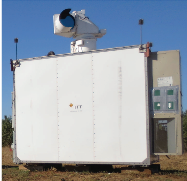
Figure 12: A more compact REAL with twice the pulse-rate of the original REAL is now available. This system is approximately 2.5 m wide by 3 m long.
