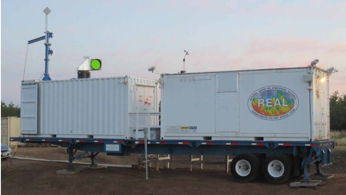
Figure 7: Photograph of the Raman-shifted Eye-safe Aerosol Lidar (REAL) at the California State University Chico farm on 23 May 2013.
