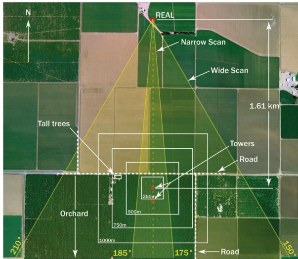
FIG. 1. Plan view of the experimental area. The yellow shaded regions from 150^{\circ} – 210^{\circ} and 175^{\circ} – 185^{\circ} azimuth represent the areas covered by wide and narrow PPI scans, respectively. The VT was located 1.61 km directly south of REAL. The white squares centered on the VT represent the outer edges of the image blocks extracted from the gridded PPI scan data that were used to compute motion vectors via the cross-correlation technique.
