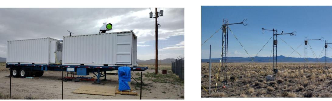
The Raman-shifted Eye-safe Aerosol Lidar (REAL) scanned horizontally at 5 m AGL and above a linear array of **50 sonic anemometers** spaced 5 meters apart at 4 m AGL. The REAL is a scanning elastic backscatter lidar at 1.54 microns wavelength. It transmits 130 mJ/pulse at 10 Hz, uses a 40 cm diameter telescope, InGaAs APDs, and a 14-bit 100 MSPS ADC. For more information on the REAL, please see:
