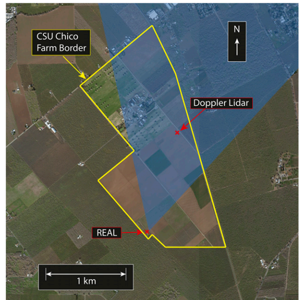
FIG. 8. A map showing the experimental setup at the University Farm at California State University, Chico, in 2013. The yellow lines represent the University Farm border. The two red symbols (×) represent the locations of the REAL system and the DL, respectively. The blue region represents the PPI scans collected by the REAL system for the experiment.
