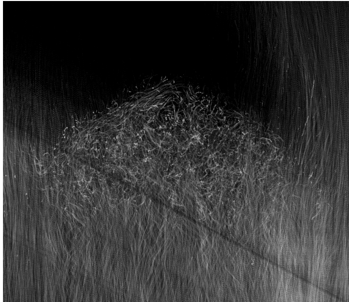
Figure 1.2: This image results from the combination (average) of 500 successive PIV frames, revealing particle trajectories – this is somehow equivalent to taking a single long-exposure shot. The dark, crescent-shaped area on the top of the picture is a sand dune – a “barchan” – viewed from above. This dune is plunged into a water stream, going downward on the picture. Left and right, almost straight particle trajectories reveal this main stream. Below (more exactly, behind) the dune, particle paths are more complex: this is the recirculation, a lower velocity region due to the shield created by the dune.
